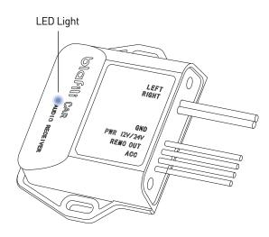
LEFT and RIGHT: Stereo RCA OUTPUT (Male) GND: POWER GROUND (INPUT) PWR: POWER +12V / +24V DC (INPUT) REMO OUT: Remote Trigger (OUTPUT) ACC: Accessory ACC (INPUT)
